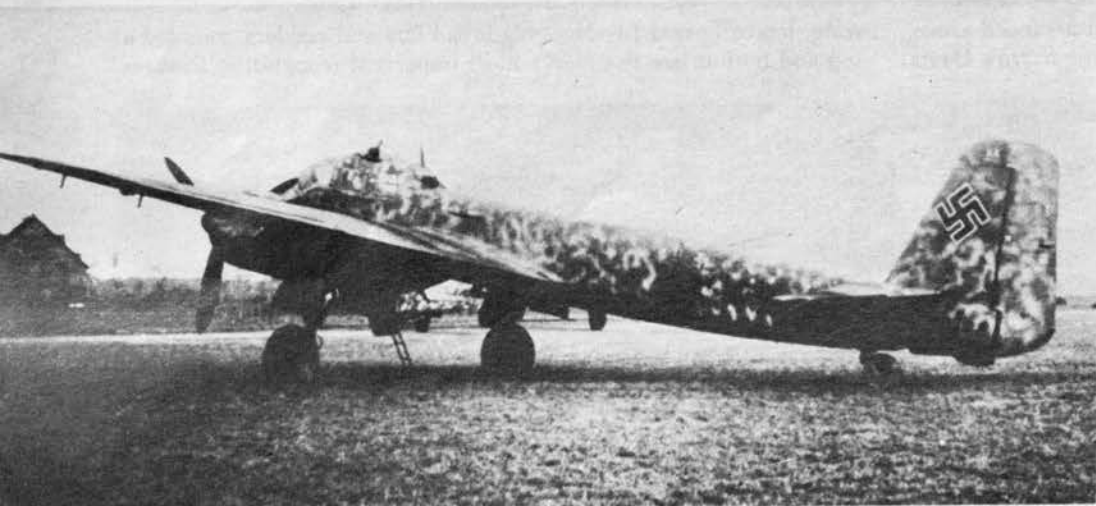
SMOOTHLY ROUNDED, GLASS-ED-IN NOSE OF JU-188 GIVES BETTER VISIBILITY. PICTURE BELOW ALSO SHOWS THE TALL UNDERCARRIAGE AND EXTREME WINGSPREAD
